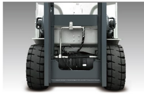
Front wheel dual drive motors offer stronger power
