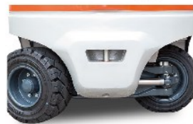
Independent steering system supplies oil for steering on demand and reduces truck energy consumption
