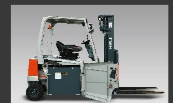
Battery side pulling changing way is easy to replace
