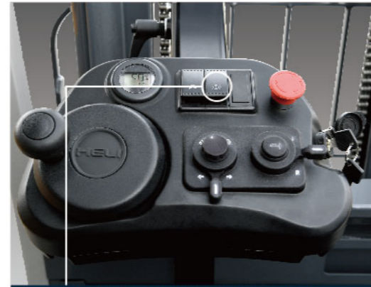
The electronic parking brake system (EPB) realizes one button parking brake and it is convenient and comfortable to operate.
