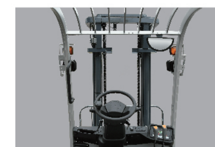
The mast with large opening offers good driving vision ensuring operation comfort and safety.
